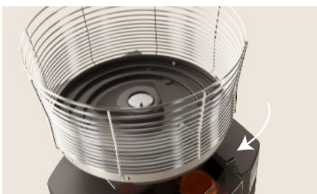
10. Place the basket in the correct position
